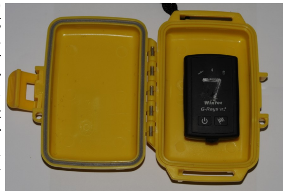
Figure 1 —Wintec™ G-Rays 2+ Global Positioning System receiver in waterproof housing
